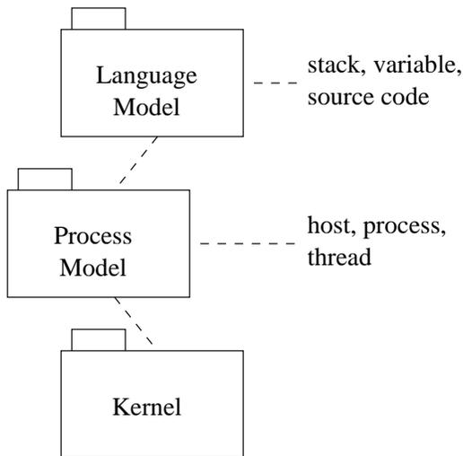
For instance, the language model, which abstracts a stack, would construct that stack's frames using register information obtained from the process model.
