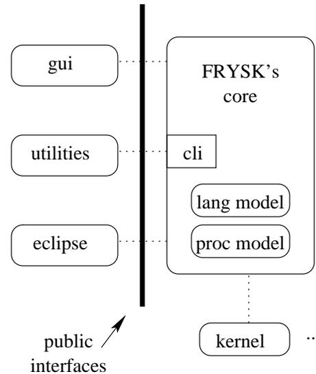
Frysk's core then uses the target system's kernel interfaces to maintain the internal models of the running system.
