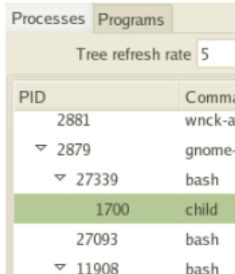
When a user requests that Frysk monitor for a process model event, such as a process exiting, that request is implemented by adding an observer (or monitor) to the objects to which the request applies. When the corresponding event occurs, the observers are notified.
