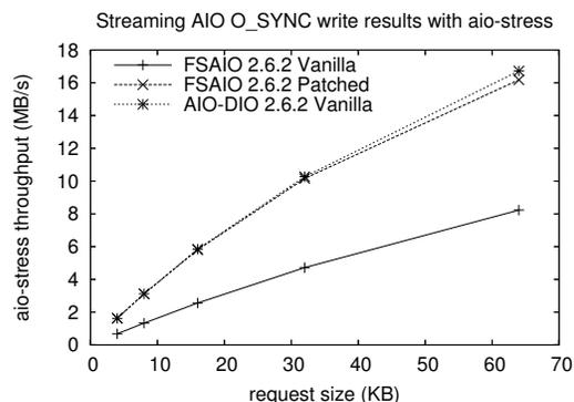
Figure 2: Comparisons of streaming random AIO write throughputs.
