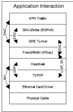
We have two Secure Gateways, each with a connection to the internet. Ideally, each would have its own link to the Internet, preferably redundant, but you could share the link if needed. Each gateway also has a connection to the local lan, which Heartbeat sends keep-alives over. If possible, use a Null-modem cable between each pair of gateways for out of band keep alives. If this isn't possible, Heartbeat also supports UDP keep-alives over any network interface.
