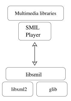
Figure 1: Basic libsmil architecture
