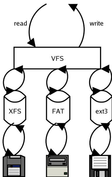
Figure 2: A diagram of the Linux VFS
