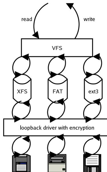
Figure 3: A diagram of the loopback encryption layer
