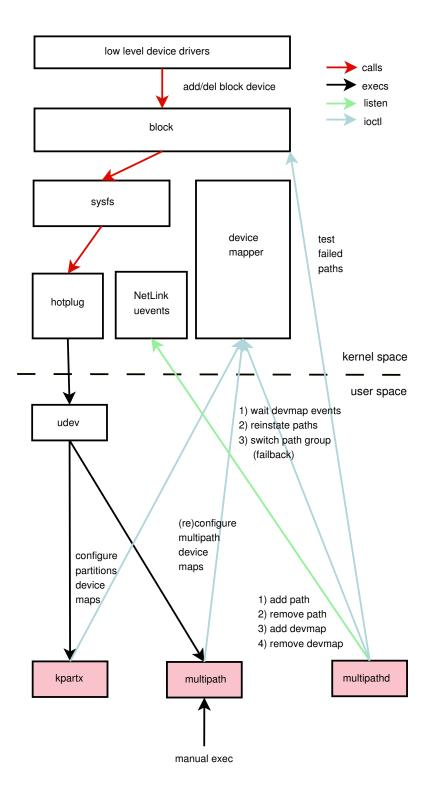
Figure 3: multipath tools architecture
